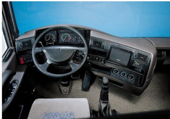
The Magnum E-Tech uses the ZF Eco-split 16 speed gearboxes with a double H gearshift pattern (more comfortable when changing gears). The Magnum E-Tech can also be fitted with the semi-automated ZF AS Tronic 16 speed gearbox.
