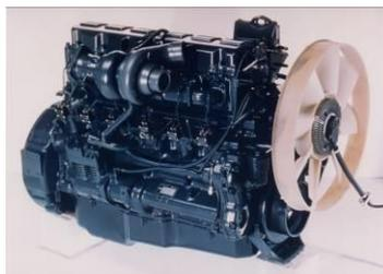
Created as the result of collaboration between the Mack design office in the United States and Renault Trucks, the development of the E-Tech 12 L engine (with power ratings of 400, 440 and 480 hp) is a significant technological step forward in terms of productivity and performance.
