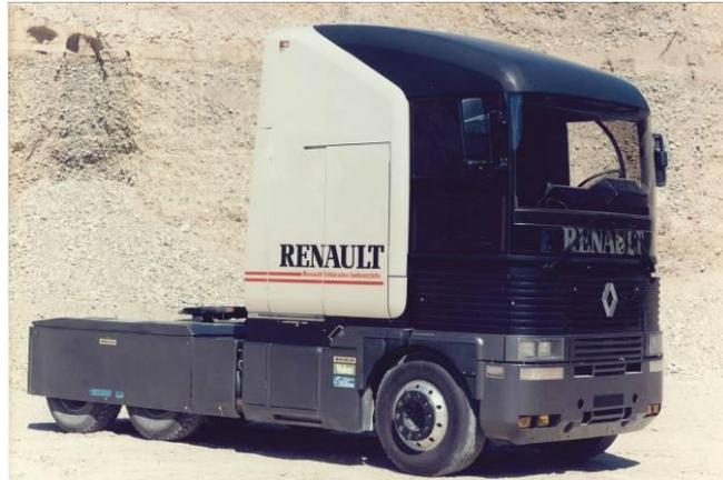
Starting in 1980, the V.I.R.A.G.E.S. program (*Véhicule industriel de recherche pour l'amélioration de la gestion de l'énergie et la sécurité* - Commercial vehicle for research into the improvement of energy management and safety) focused on studying a certain number of technical options designed to be featured in future production vehicles. This program resulted in the building of two VE (experimental vehicle) prototypes, named the VE 10 (1985) and the VE 20 (1988).
